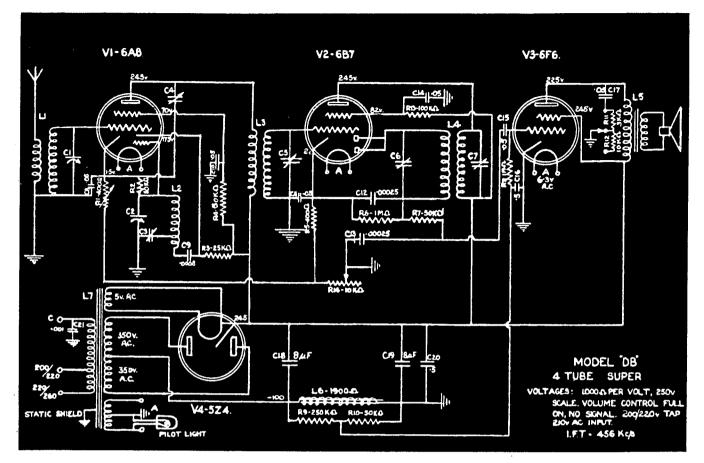
Astor model "55," chassis type "DB," is a four-valve receiver designed for broadcast coverage and operation from 200-260 volts A.C. mains. This receiver is of the console type and is fitted with three controls-volume, tuning, tone (3 positions)—and an 8 inch, 1,900 ohms field,
