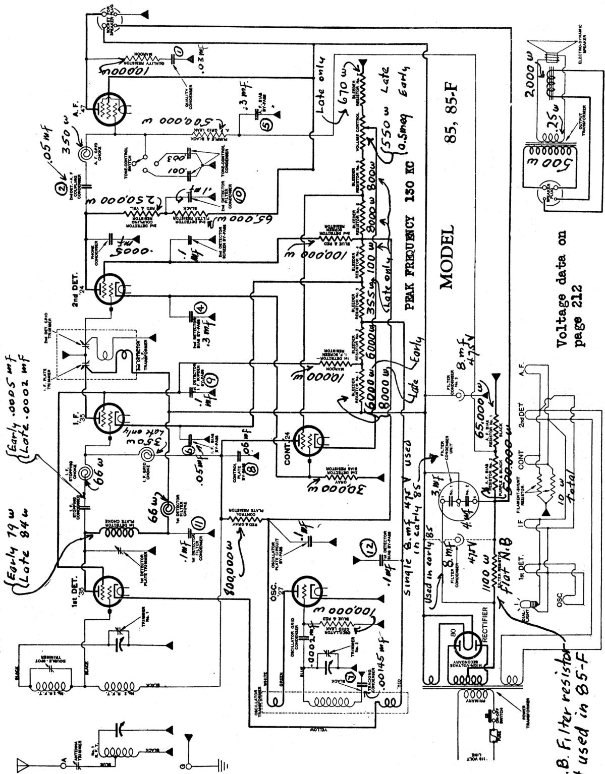
A few early-type Model 85 do not have automatic volume control; they have three electrolytic filter condensers; the circuit of these early Model 85 sets is similar to Model 80. The tracking condenser is mounted on the oscillator transformer in Model 82 and some 85 sets. The filament circuit of Model 82 is somewhat different from that shown above.
