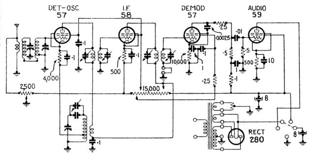
Tasma model "135" is a five-valve, A.C. operated, broadcast receiver which dates back to 1933. This model is housed in a console type cabinet and has a dial of the "travelling light" type. The dial lamp is a 2.5 volt, miniature-screw type. Only two controls are fitted, these being for tuning and volume. The latter is of the "R.F." type which simultaneously controls the aerial input and I.F. amplifler gain, and is wired so that the bleed current of the voltage divider passes through it to earth.
