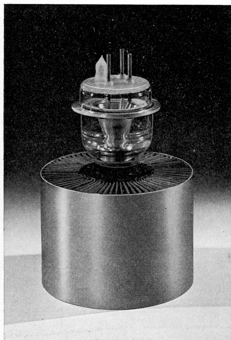
Fig. 2c. Triode with thoriated tungsten heater: TBL 6/6000. The anode of this valve is forced-air cooled.
