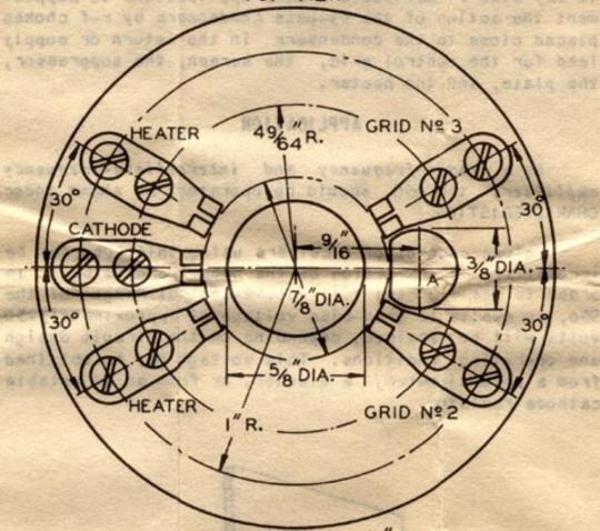
1/4 HIGH A = ALIGNMENT PLUG NOTE: INSERT TUBE IN CLIPS SO THAT SHORT END OF TUBE RESTS IN THE MOUNTING HOLE
