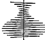
AMPLITUDE-MODULATED RF WAVE
