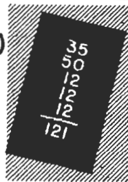
FILAMENTS IN SERIES (UNIVERSAL A.C.-D.C. SET)
