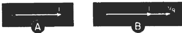
FIG. 25. The starting or reference position is shown at A. Each complete revolution of a vector represents one a.c. cycle. By general agreement among radio and electrical men, vectors are always assumed to be rotating counterclockwise, opposite to the direction in which the hands of a clock move. Furthermore, the starting or reference position for all vectors is the vector position shown at A, which is a line going to the right horizontally from the center (O) of the vector diagram. In a series circuit, we almost always use current for our reference vector. To make the vector A represent the circuit current, we make the length of the vector proportional to the effective current value which would be indicated by an a.c. ammeter. We then put on the arrow head, and label it with the capital letter I to indicate that it represents current. As the resistor voltage drop is in phase with the current, its position will be the same as the reference line, so we draw it right on top of the current line, as at B.
