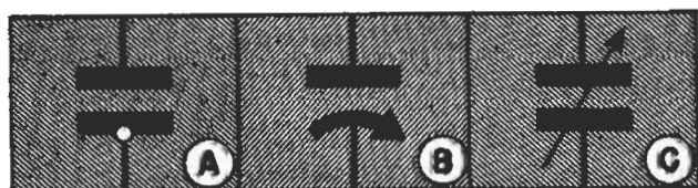
FIG. 13. Adjustable condenser symbols used in wiring diagrams. The one at A is used for trimmer condensers. The other two are used for variable tuning condensers usually, although sometimes they are used to indicate trimmers too.
