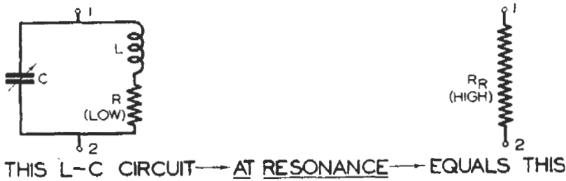
FIG. 8. A coil-condenser load (a parallel resonant circuit) acts as a resistor of high ohmic value at the resonant frequency of the circuit.
