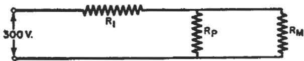
FIG. 25. Notice how the voltmeter resistance is in parallel with the tube plate-cathode resistance.
