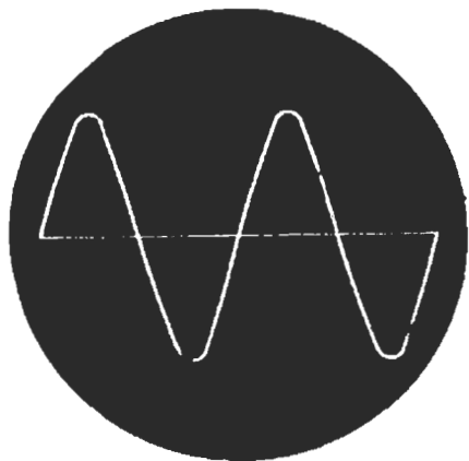
FIG. 33. When the sweep frequency is half the vertical deflecting frequency, two cycles will be produced.
