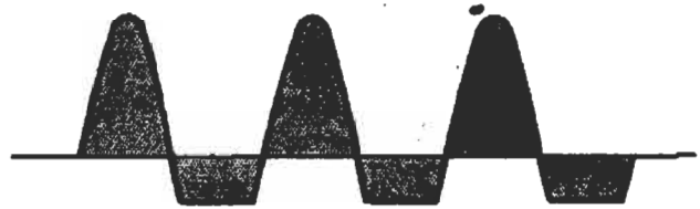
FIG. 18. A distorted wave, such as might be produced by operating a tube at the wrong point on the characteristic.
