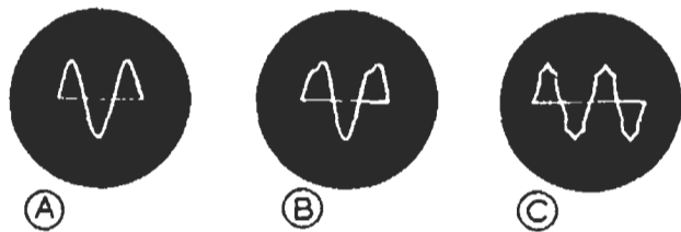
FIG. 1. These diagrams, copied from curves produced on the screen of a cathode ray oscilloscope in the N. R. I. laboratory, show what happens when a selective radio receiver is carelessly tuned. At A is the audio output curve secured when the receiver is correctly tuned to a carrier modulated with a single pure sine wave; there is no distortion. The slightly-distorted audio output wave form produced when the receiver is tuned about 2 kc. above the input R.F. carrier frequency appears at B, while the severely distorted wave form at 10 kc. off-tune appears at C.
