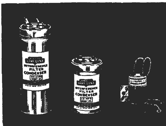
FIG. 5. Typical interference elimination units. Left to right: Sprague Type IF-11 dual 1 mfd., 600 volt condenser with metal can serving as common terminal; Sprague Type IF-50 single 1 mfd., 1,000 volt condenser unit with two terminals; Sprague Type IF-33, 1,000 volt rating condenser with two flexible leads, available in two capacities; Sprague Type CH-1 special interference eliminating choke coil (above), rated to carry 10 amperes and mounted in a metal case which should always be grounded.
