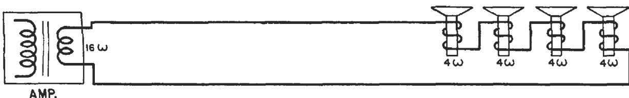
FIG. 14. Matching impedances of series-connected voice coils.
