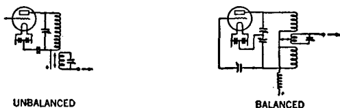
Figure 20. Showing How Coupling for an End-Fed Antenna May Be Accomplished
