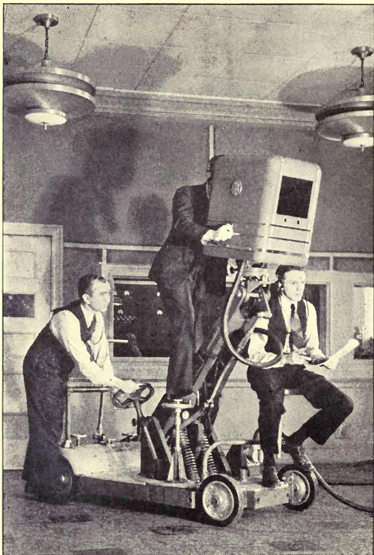
FIG. 36—Television Camera mounted on a dolly. A studio crew in action at the General Electric Company.
