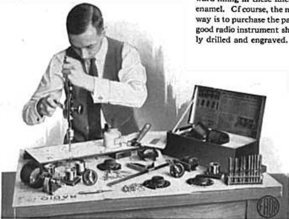
Showing "Neutrodome" receiver panel in the process of being drilled, using the paper template supplied with this book.
