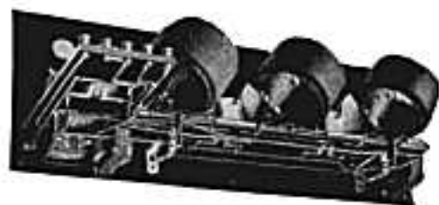
Interior view of the "One-Sixty" Hazeltine Neutrodyne receiver showing arrangement of wiring and "Neutroformer" units.
