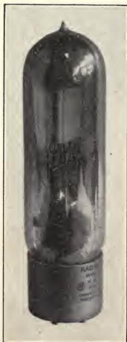
Fig. 74. — Illustrating Radiotron; UV-203; a 50-watt power tube.
