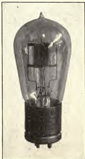
Fig. 75.—Illustrating 5-watt Radiotron; UV-202.
