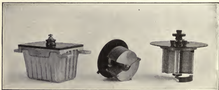
Fig. 13.—Types of condensers for radio circuits: (a) Mica condenser for transmitting circuits; (b) and (c) variable condensers for receiving circuits.
