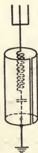
Fig. 77.—Showing method of reducing dielectric losses by surrounding antenna coil and grid condenser with a grounded metal screen.
