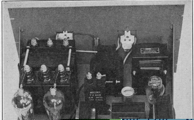
Figure 20. This chassis contains a 350-volt power supply and a 1250-volt power supply. Low-voltage power supply components are to
