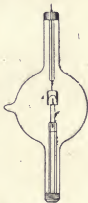
FIG. 42.—Small Kenotron or High-Vacuum Fleming Oscillation Valve as made by the General Electric Company of America.
