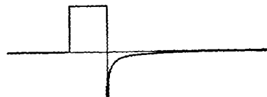
FIG. 3-25.—Spike often produced by shunt capacity.
