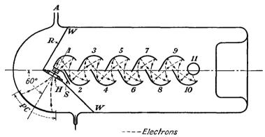
Fig. 19.14.—Structure of a partition-type photomultiplier tube.
