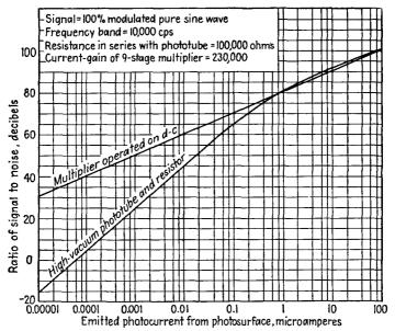
Fig. 19.18.—Comparative signal-to-noise ratios of a photomultiplier tube and a vacuum phototube with amplifier.
