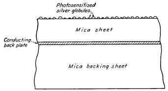
Fig. 20.33.—Structure of the iconoscope mosaic.
