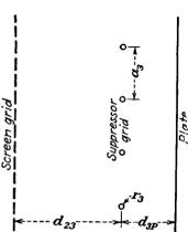
Fig. 11.8.—Electrode dimensions in the suppressor-grid region.
