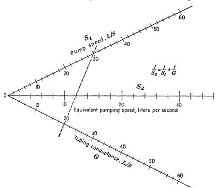
Fig. 21.25.—Nomographic chart of equivalent pump speed.
