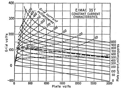
Fig. 9.3.—Contours of constant plate current.
