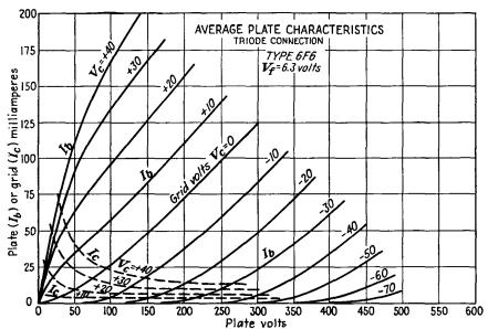
Fig. 9.2.—Plate-current-plate-voltage characteristics of a triode.
