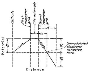
Fig. 17.29.—Potential profiles of a reflex-klystron oscillator.
