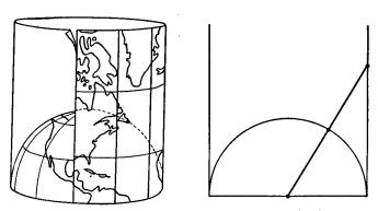
Fig. 5.22.—Construction of the Mercator projection.
