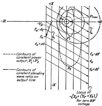
Fig. 18.30.—Locus of  $-[Z_l + \omega^2 M^2(Y_r + Y_s)]$  in an impedance plane.
