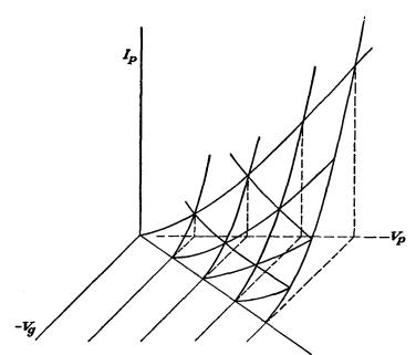
Fig. 9.4.—The plate-current surface.
