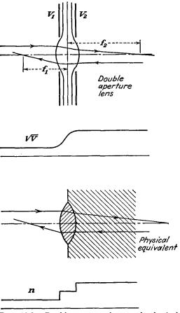
Fig. 13.3.—Double-aperture lens and physical equivalent.
