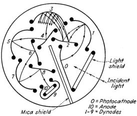
Fig. 19.17.—Structure of a circular photomultiplier tube.
