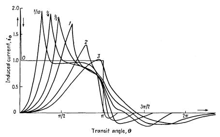
Fig. 16.23.—Induced-current pulses in an unbiased diode without space charge.
