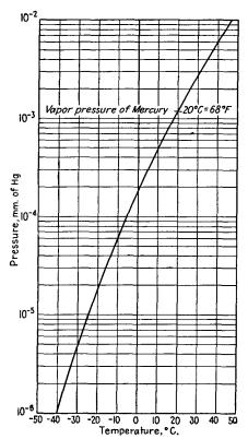
Fig. 21.30.—Vapor pressure of mercury as a function of temperature.
