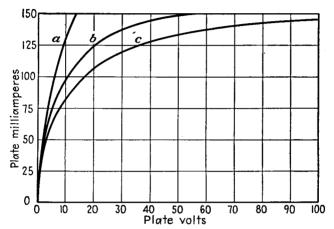
Fig. 11.19.—Plate-current-plate-voltage characteristic of a tube with electrons scattered by one, two, or three grids.
