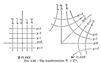
tion of points is used the angle of the point in the W plane is half the angle of the corresponding point in the Z plane and the radius vector of a point in the W plane is the square root of the radius vector of the corresponding point in the Z plane.
