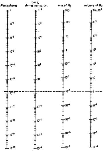
Fig. 21.1.—Comparison of pressure scales.
