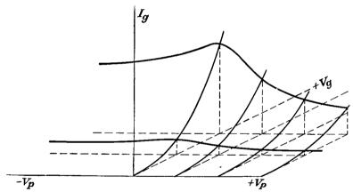
Fig. 9.14.—The grid-current surface.
