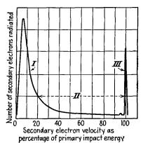
Fig. 4.17.—The relative velocity distribution of secondary electrons. About 90 per cent of the secondary electrons will have velocities in range I, 7 per cent in range II, and 3 per cent in range III.
