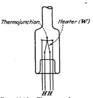
Fig. 21.18.—Thermocouple vacuum gauge.
