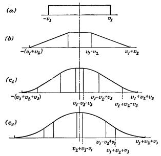
Fig. 11.18.—Distribution of sidewise component of velocity in a beam of electrons scattered by one, two, or three grids.
