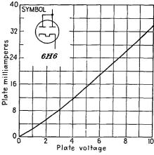
Fig. 2.1.—Plate-current—plate-voltage characteristics of a diode.
