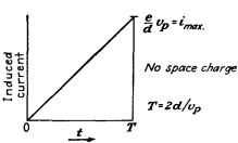
16.6.—Induced current resulting Fig. from an electron in transit in a parallelplane diode without space charge.
