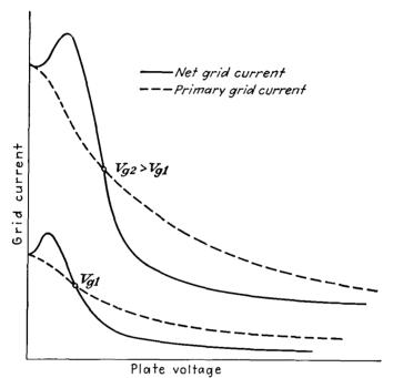
Fig. 9.16.—Influence of secondary emission upon the grid-current-plate-voltage characteristics of a triode.
