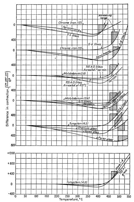
Fig. 21.40.—Difference in contraction of the principal sealing glasses and metals.
