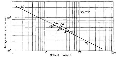
Fig. 21.3.—Average velocity of gases at room temperature.
