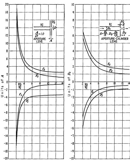
Fig. 13.33.—Optical characteristics of a double-aperture lens, A/D=1.
