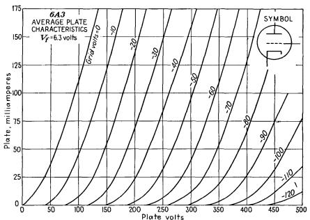
Fig. 2.2.—Plate-current—plate-voltage characteristics of a triode.
