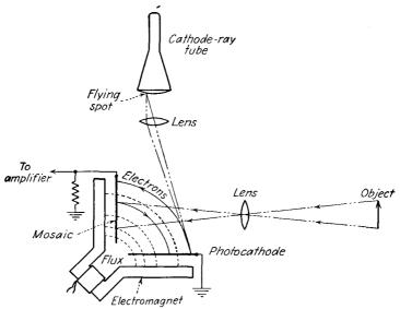
Fig. 20.35.—Structure of the orthicon.
