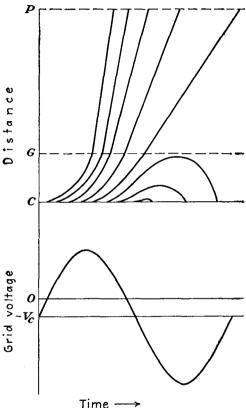
Fig. 16.24.—Distance-time diagram of electrons in a triode.
