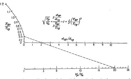
Fig. 16.21.—Nomographic chart relating triode transit times in the presence of space charge to electrode dimensions and voltages as given by Eq. (16.75).
