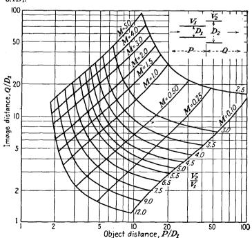
Fig. 13.39.—P-Q curves of a two-cylinder lens,  $D_2/D_1 = 1.5$ , 379
