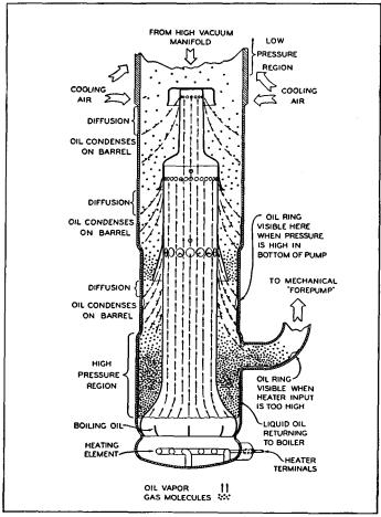
Fig. 21.34.—Air-cooled oil-vapor pump. (Eimac HV1.)
