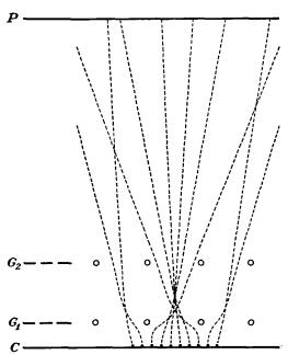
Fig. 10.6.—Electron paths in a beam-power tube. (Jonker.)
