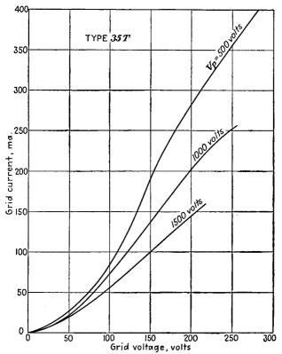
Fig. 9.12.—Grid-current—grid-voltage characteristics of a type 35T triode.
