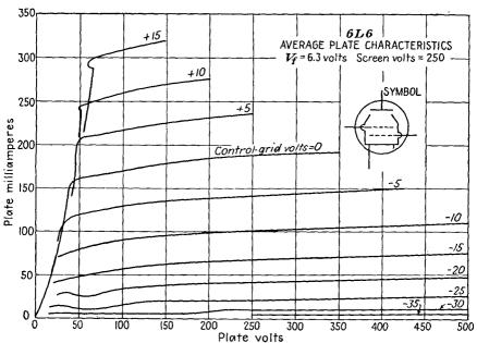
Fig. 2.7.—Plate-current—plate-voltage characteristics of a beam-power tube.
