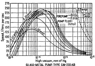
Fig. 21.37.—Operating characteristics of a three-stage fractionating pump.
