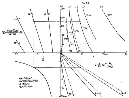
Fig. 17.45.—Construction of a reflector-voltage-cavity-length plot.
