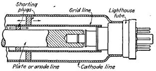
Fig. 16.29.—Double concentric-line oscillator utilizing a lighthouse tube.
