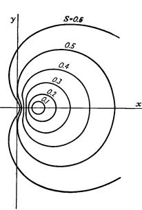
Fig. 7.9.—The shape of large transformed grid wires in the Z-plane representation of Fig. 7.1. The transformed grid wires are nearly circular for screening fractions as large as 0.2. Beyond this value, the grid contour is noncircular and cannot be represented by two line charges.
