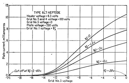
Fig. 20.11.— $I_p$ - $V_3$  characteristics of the heptode.
