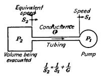
Fig. 21 24.—Diagram illustrating equivalent pumping speed.
