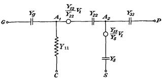
Fig. 16.15.—Equivalent circuit of a tetrode at ultra-high frequencies.
