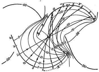
Fig. 19.15.—Electron paths in the partition-type photomultiplier tube.
