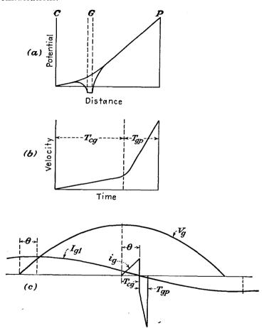
Fig. 16.9.—Factors determining induced grid current in a plane-electrode triode.
