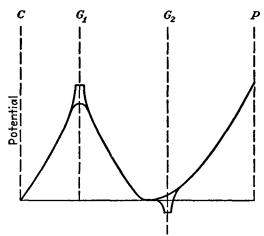
Fig. 20.17.—Potential profiles in the space-charge-grid triode.
