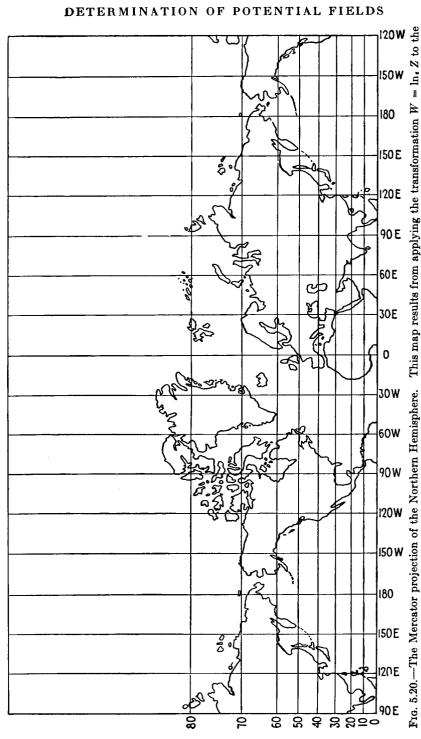
This map results from applying the transformation  $W = \ln \epsilon Z$  to the polar azimuthal equidistant projection of Fig. 5.19.
