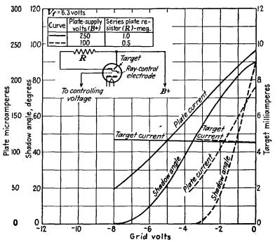
Fig. 20.24.—Triode-ray-tube characteristics.
