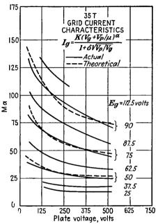
Fig. 9.20.—Comparison of actual and theoretical grid current.
