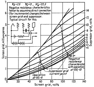
Fig. 20.19.—I<sub>2</sub>-V<sub>2</sub> characteristics of a pentode.
