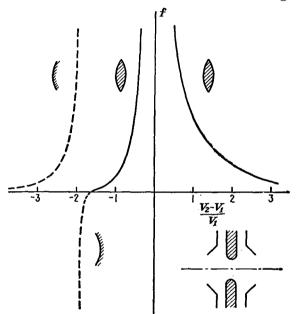
Fig. 13.49.—Focal characteristics of an Einzel lens.
