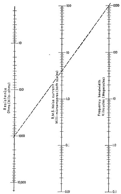
Fig. 12.3.—Nomographic chart of equivalent rms current through a noisy resistor.
