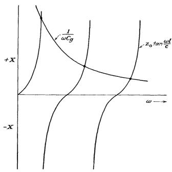
Fig. 17.42.—Curves of reflex-klyst on gap reactance and inductive line reactance as a function of frequency.
