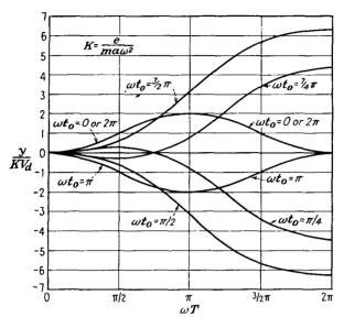
Fig. 15.39.—Path of an electron between deflecting plates when the transit time is large compared to the period of the deflecting voltage.
