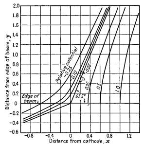
Fig. 15.25.—Potential field required to produce a parallel-flow rectangular beam.
