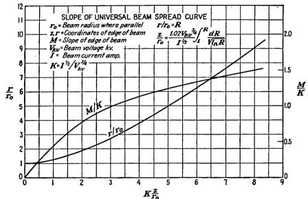
Fig. 15.38.—Slope of universal beam-spread envelope.
