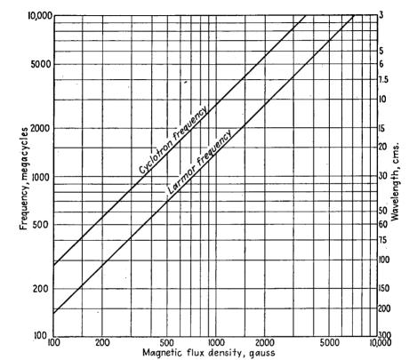
Fig. 18.11.—Dependence of the cyclotron and Larmor frequencies upon the magnetic-flux density.
