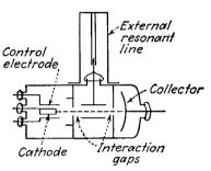
Fig. 17.54.—Diagram of the Heil tube.
