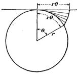
Fig. 5.21.—Construction of the polar azimuthal equidistant projection.
