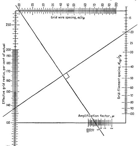
Fig. 9.21.—Nomograph of effective grid radius.
