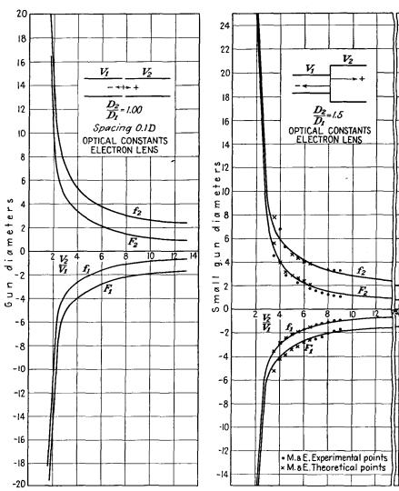
Fig. 13.27.—Optical characteristics of a two-cylinder lens,  $D_2/D_1 = 1$ .
