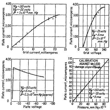
Fig. 21.20.—Characteristics of a typical triode ionization gauge.
