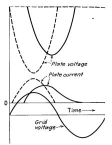
Fig. 16.25.—Distortion of the plate-current pulse in a Class C triode amplifier caused by transit-time effects.
