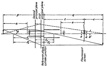
Fig. 13.24.—Experimental determination of electrostatic lens characteristics.
