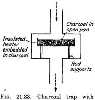
Fig. 21.33.—Charcoal trap with electric heater.
