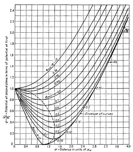
Fig. 10.10a.—Potential-distribution curves of the type C.
