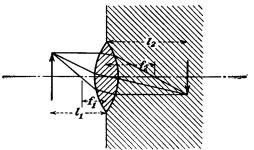
Fig. 13.6.—Focal relations in a lens operating between two different media.
