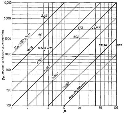
Fig. 9.8.—Constants of typical triodes.
