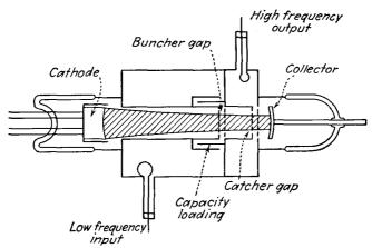
Fig. 17.23.—Structure of the frequency-multiplier klystron.
