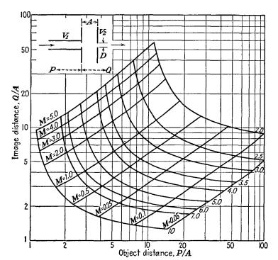
Fig. 13.42.—P-Q curves of a double-aperture lens,  $A/D \approx 5$ .
