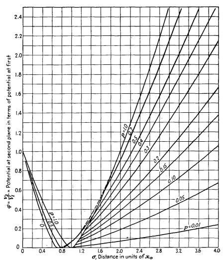
Fig. 10.9.—Potential-distribution curves of the type B.
