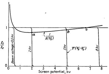
Fig. 15.16.—Graphical construction of the screen-potential-beam-potential characteristic,
