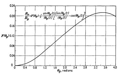
Fig. 17.20.—Theoretical equivalent bunching resistance of a beam as a function of the intergrid transit angle. (After Feenberg.)
