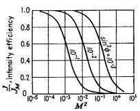
Fig. 15.18.—Intensity efficiency of an electron gun as a function of cathode magnification for various aperture
