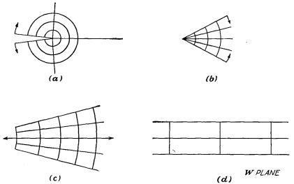
Fig. 5.18.—Steps in a progressive transformation from the Z to the  $\ln_\epsilon Z$  plane.
