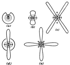
Fig. 20.25.—Directed-ray electron-tube structures.
