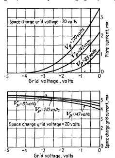
Fig. 20.18.—Current-voltage characteristics of the space-charge-grid triode.
