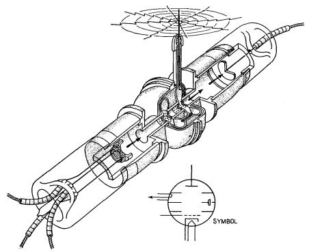
Fig. 2.9.—Cutaway view of a two-resonator klystron oscillator.
