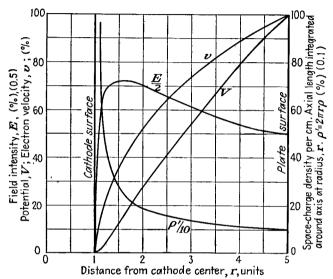
Fig. 8.6a.—Curves of potential, gradient, space-charge density, and velocity as a function of radial distance in a space-charge-
