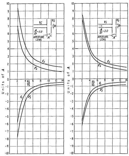
Fig. 13.31.—Optical characteristics of a double-aperture lens, A/D=5.
