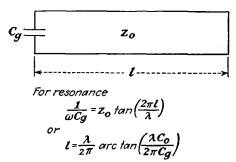
Fig. 17.41.—Equivalent circuit of a concentric-line resonator and reflex-klystron oscillator.
