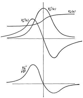
Fig. 13.17.—Axial potential functions of a double-aperture lens.
