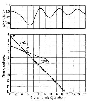
Fig. 16.14.—Small-signal transadmittance of a triode as a function of cathode-grid transit angle. (After Liewellyn.)
