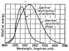
Fig. 15.13.—Spectral characteristics of willemite.
