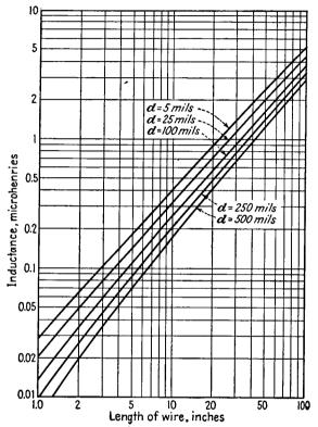
Fig. 16.1.—Inductance of a round straight wire.
