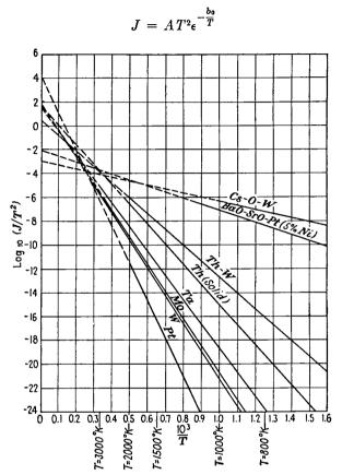
Fig. 4.5.—Characteristics of the common emitters shown as a curve of  $\log J/T^2$  against 1/T. This type of plot demonstrates the validity of the Richardson-Dushman equation (4.3). The y-axis intercepts give the emission constant A. The slope of the lines is proportional to the work function of the emitter.
