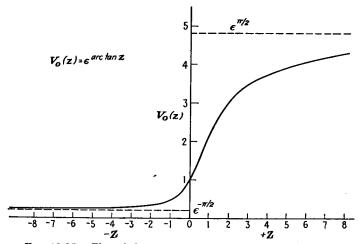
Fig. 13.35.—Plot of the axial potential,  $V_0(z) = \exp (\arctan)$ .
