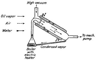
Fig. 21.32.—Typical glass, water-cooled, oil-diffusion pump.
