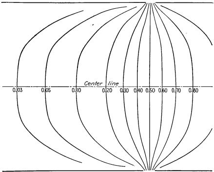
Fig. 13.8.—Field plot of an equal-diameter two-cylinder lens.
