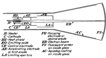
Fig. 15.1.—Schematic cathode-ray-tube structure.
