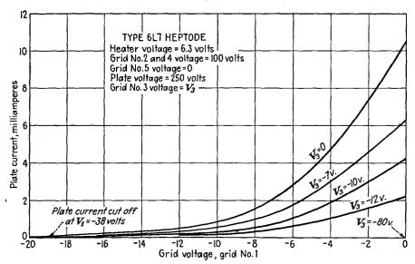
Fig. 20.10.— $I_p$ - $V_1$  characteristics of the heptode.
