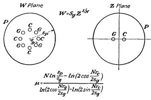
Fig. 7.19c.—The amplification factor of a cylindrical triode whose cathode is a group of wires located between the wires of a squirrel-cage grid.
