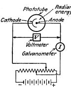
Fig. 19.1.—Circuit for observing the photoelectric effect.
