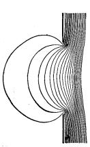
Fig. 13.15.—Potential field of a single-aper-ture lens.
