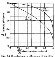
Fig. 15.19.—Intensity efficiency of an electron gun as a function of current efficiency.
