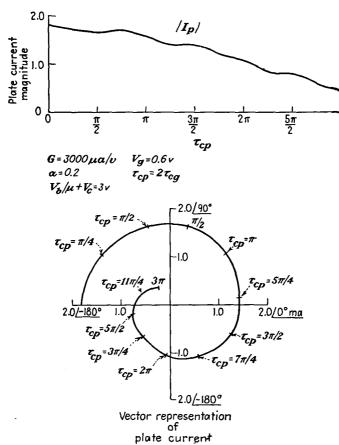
Fig. 17.55.—Triode plate current as a function of transit angle for relatively small excitation.
