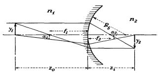
Fig. 15.7.—Spherical-surface refraction equivalent of cathodelens action.
