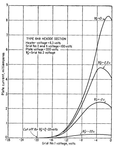
Fig. 20.2.— $I_p$ - $V_1$  characteristics of a hexode.
