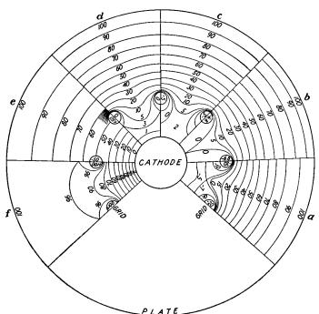
Fig. 7.6.—Equipotential contours in the cylindrical-electrode triode:
