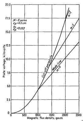
Fig. 18.24.—Mode lines in the voltage-magnetic-flux-density plane,
