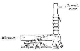
Fig. 21.36.—Diagram of two-stage fractionating pump.
