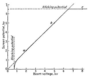
Fig. 15.17.—Screen-potential-beam-potential characteristic of a fluorescent screen.
