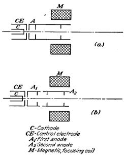
Fig. 15.9.—Electron guns with magnetic focusing.
