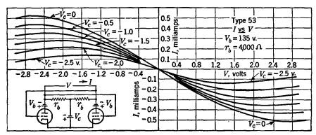
Fig. 20.20.—Current-voltage characteristics of the push-pull circuit.
