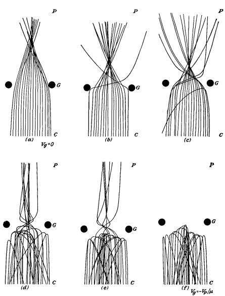
Fig. 9.10.—Electron paths in a negative-grid triode (Kleynen).
