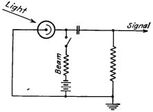
Fig. 20.31.—Equivalent circuit of a mosaic picture element.
