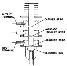
Fig. 17.21.—Structure of the cascade amplifier.
