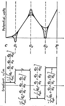
Fig. 11.10.—Potentials and gradients in a pentode.
