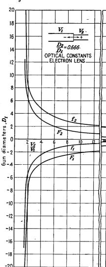
Fig. 13.26.—Optical characteristics of a two-cylinder lens,  $D_2/D_1 = 2/3$ .
