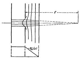
Fig. 13.19.—Convergent action of a single-aperture lens.
