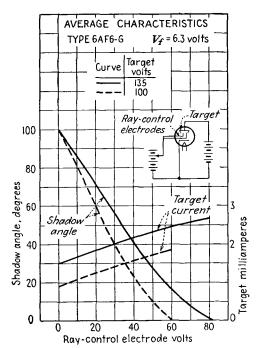
Fig. 20.23.—Electron-ray-tube characteristics.
