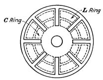
Fig. 18.10.—Inductive and capacitive tuning rings.
