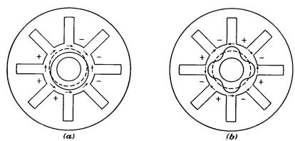
Fig. 18.5.—Fields in multicavity magnetrons.
