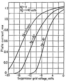
Fig. 11.4.—Plate-current-suppressor-grid characteristics of a type 6J7 pentode.
