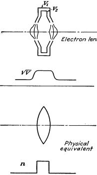
Fig. 13.2.—Electron lens equivalent of a thin physical lens.
