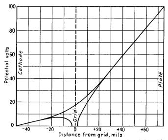
Fig. 7.4d.—Potential profiles in a plane-electrode triode, with grid at zero potential,
