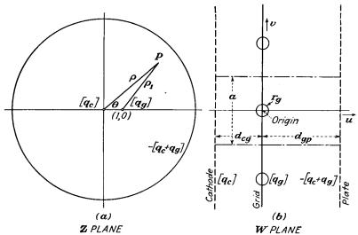
Fig. 7.1.—Elementary triode and equivalent plane-electrode triode.
