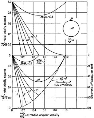
Fig. 18.21.—Total and radial electron velocity at the anode of a magnetron as a function of magnetic-flux density and angular velocity for a small ratio of cathode to plate radius. (After Posthumus.)
