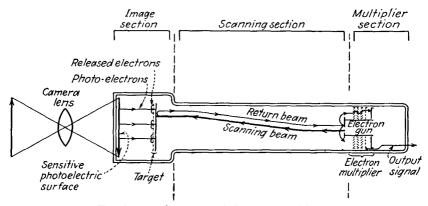
Fig. 20.36.—Structure of the image orthicon.
