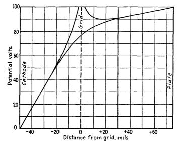
Fig. 7.4e.—Potential profiles in a plane-electrode triode, with grid and plate at the same positive potential. This condition may exist at the peak of the current pulse in a Class C amplifier.
