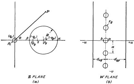
Fig. 7.10. -W- and Z-plane representations of a high-mu plane-electrode triode. This is the basis of the analysis of Vodges and Elder.
