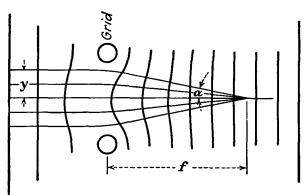
Fig. 11.16.—Focal action of a grid.
