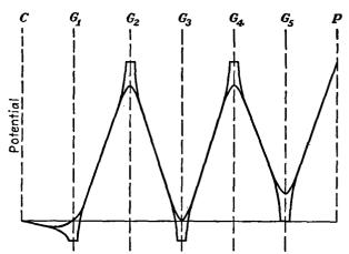
Fig. 20.9.—Potential profiles of the heptode.
