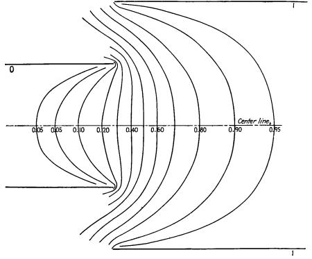
Fig. 13.12.—Potential field of a two-cylinder lens,  $D_2/D_1 = 2.0$ .
