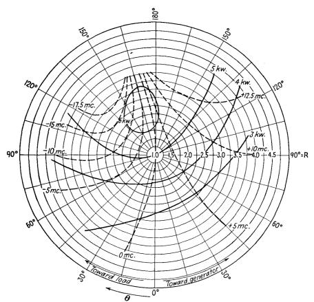
Fig. 18.31.—Rieke diagram of a Raytheon 2J38 magnetron.
