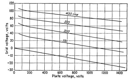
Fig. 8.8.—Constant-current representation of triode characteristics.
