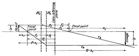
Fig. 13.21.—Graphical construction of a thick-lens image.
