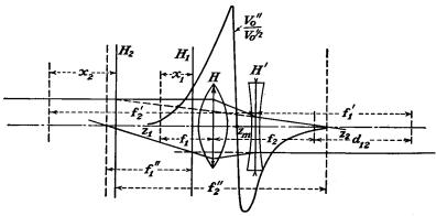
Fig. 13.23.—Thin-lens components of a thick lens.
