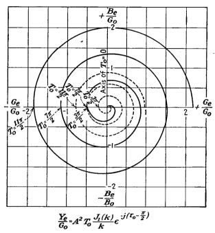
Fig. 17.34.—Electronic-admittance spirals of reflex-klystron oscillators.
