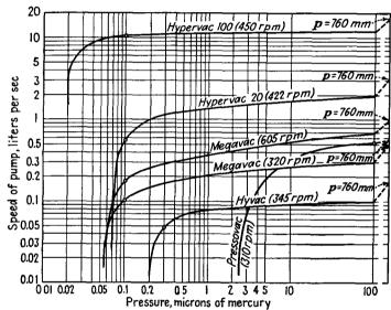
Fig. 21.27.—Speed-pressure curves of mechanical vacuum pumps.
