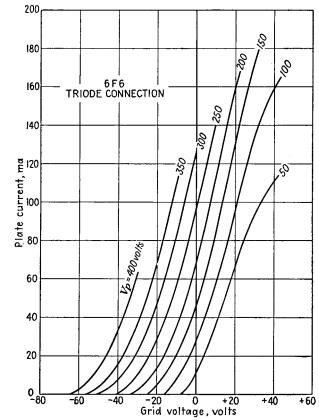
Fig. 9.1.—Plate-current-grid-voltage characteristics of a triode.
