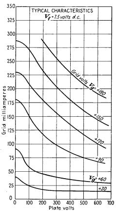
Fig. 9.13.—Grid-current-plate-voltage characteristics of a type 826 triode.
