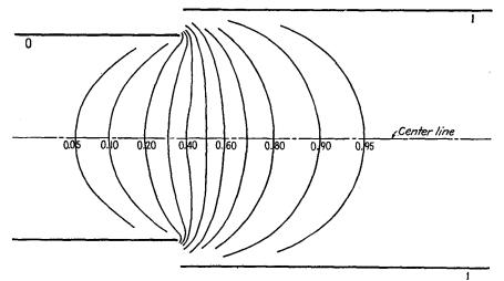
Fig. 13.10.—Potential field of a two-cylinder lens,  $D_2/D_1 = 1.25$ .
