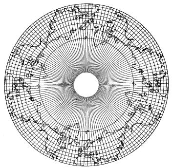
Fig. 5.25—Polar azimuthal equidistant projection of the Northern Hemisphere transformed by  $W = Z^{\frac{1}{2}}$ .
