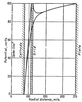
Fig. 7.7e.—Potential profiles in a cylindrical triode, with grid and plate at equal positive potentials.
