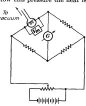
Fig. 21.14. — Constant-resistance method of using the Pirani gauge.
