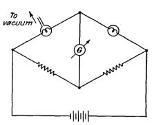
Fig. 21.16.—Pirani gauge with bridge unbalance indicator.
