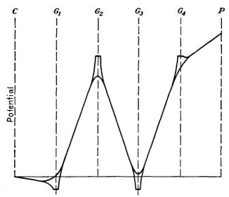
Fig. 20.1.—Potential profiles in a hexode.
