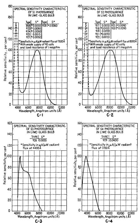
Fig. 19.9.—Spectral response curves of typical RCA phototubes.
