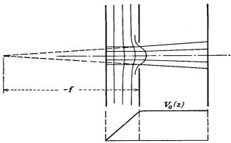
Fig. 13.18.—Divergent action of a single-aperture lens.
