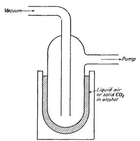
Fig. 21.29.—Freezing trap for collecting condensable vapors.
