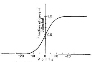
Potential difference between collector and screen Fig. 15.15.—Collector current of a cathode-ray tube as a function of the difference of collector and fluorescent-screen potential.
