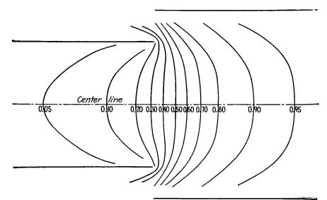
Fig. 13.11.—Potential field of a two-cylinder lens,  $D_2/D_1 = 1.5$ .
