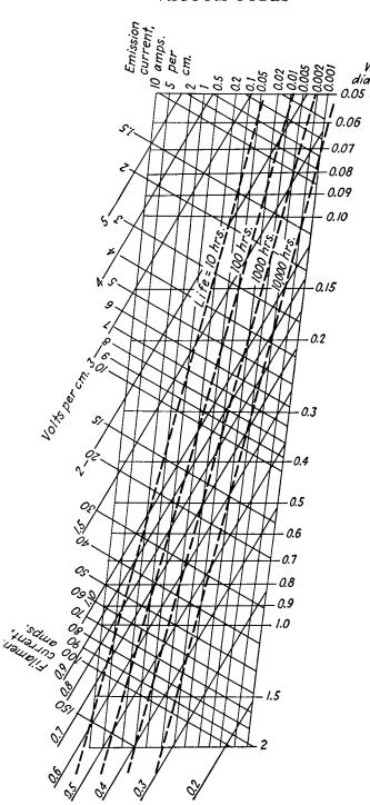
Curves are for a 1-cm length of wire, Fig. 4.10.—Characteristics of ideal tungsten filaments as given by the data of Langmuir and Jones. Life is defined as the time required for a 10 per cent reduction in mass through evaporation.
