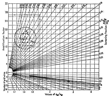
Fig. 7.12.—Amplification factor of a cylindrical triode.
