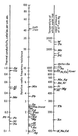
metals used in vacuum-tube construction.
