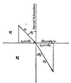
Fig. 13.1.—Electron refraction.
