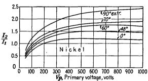
Fig. 4.19.—Variation of secondary-emission ratio with angle of primary impact. Note that the secondary-emission ratio increases as the angle of incidence becomes more nearly grazing. (After Bruining and DeBoer.)
