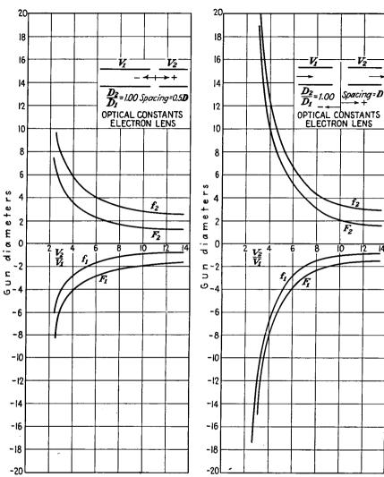
Fig. 13.29.—Optical characteristics of an equal-diameter two-cylinder lens, S = 0.5D.
