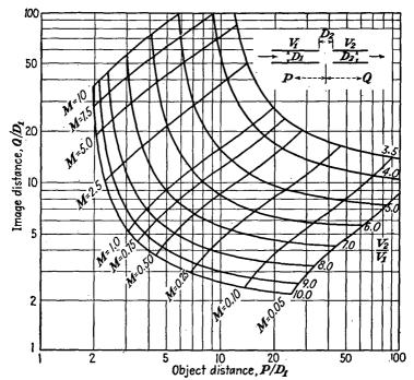
Fig. 13.41.—P-Q curves of a two-cylinder lens,  $D_2/D_1=1$ ,  $S=1.0D_1$ . 380
