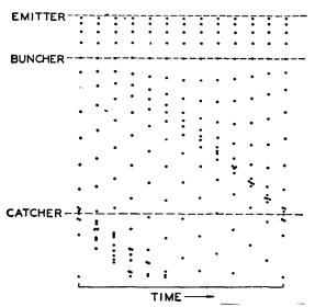
Fig. 17.1.—Elementary representation of bunching action.
