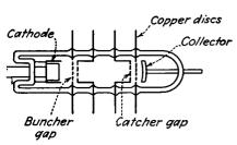
Fig. 17.17.—External-cavity klystron amplifier.
