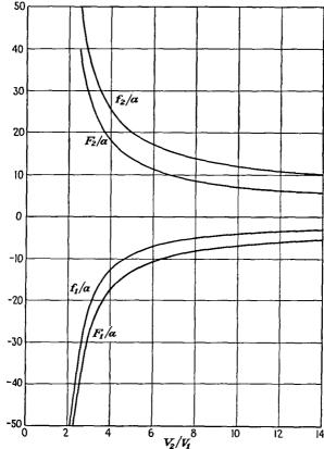
Fig. 13.36.—Optical characteristics of the Hutter lens.
