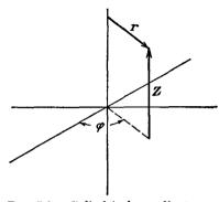
Fig. 5.8.—Cylindrical coordinate notation.
