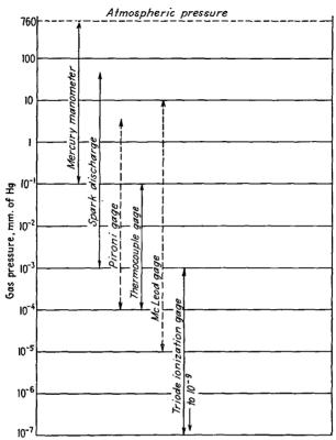
Fig. 21.9.—Range of various pressure-measuring devices.
