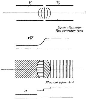
Fig. 13.4.—Two-cylinder lens and physical equivalent.
