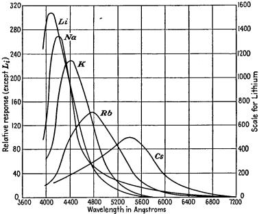
Fig. 19.6.—Photoelectric color sensitivity of the alkali metals.
