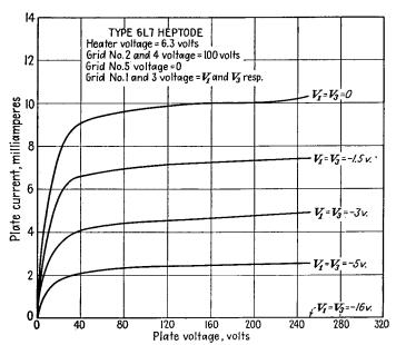
Fig. 20.12.— $I_p$ - $V_p$  characteristics of the heptode.
