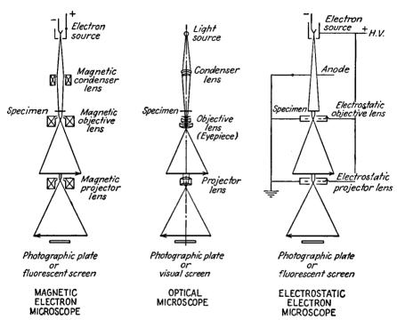
Fig. 20.37.—Structure of the electron microscope.
