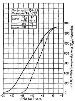
Fig. 20.13.— $g_{1p}$ - $V_3$  characteristics of the heptode.
