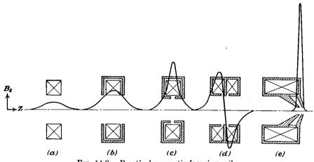
Fig. 14.8.—Practical magnetic focusing coils.
