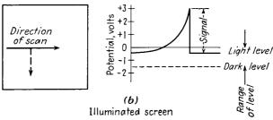
Fig. 20.32.—Potential reaction of mosaic to scanning.
