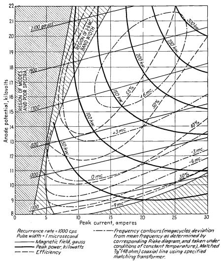
Fig. 18.32.—Voltage-current characteristics of a Raytheon 2J30 magnetron.
