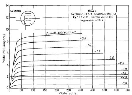
Fig. 2.4.—Plate-current—plate-voltage characteristics of a pentode.
