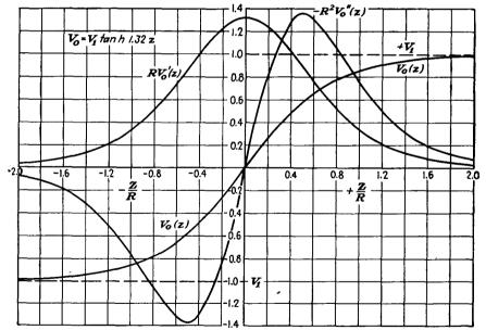
Fig. 13.9.—Axial potential and its derivatives—equal-diameter two-cylinder lens.
