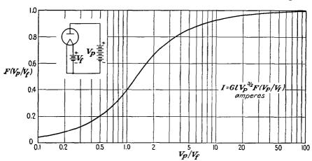
Fig. 8.11.—Filament voltage-drop emission correction factor.
