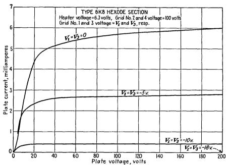
Fig. 20.4.— $I_p$ - $V_p$  characteristics of a hexode.
