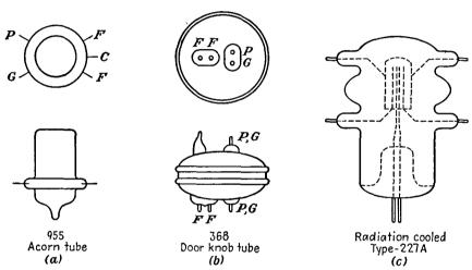
Fig. 16.3.—Common ultra-high-frequency tube types.
