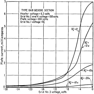
Fig. 20.3.— $I_p$ - $V_3$  characteristics of a hexode.
