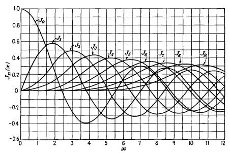
Fig. 17.13.—Curves of the higher order Bessel functions.
