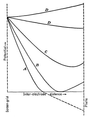
Fig. 10.7.—Types of potential distributions in the screen-grid-plate region of a beam-power tube.
