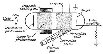
Fig. 20.34.—Structure of the image iconoscope.
