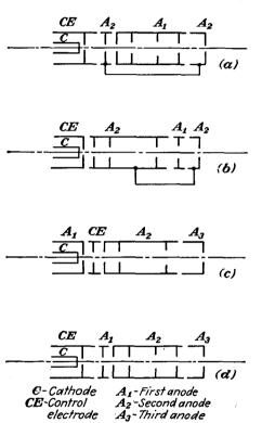
Fig. 15.8.—Typical electron-gun structures using electrostatic focusing.
