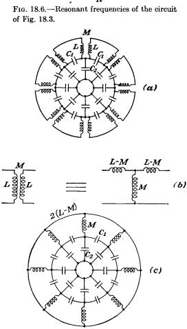
Fig. 18.7.—Equivalent circuits of multicavity magnetrons including the mutual inductance between slots.
