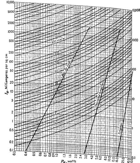
Fig. 4.7.—Emission-current density as a function of heating power for typical examples of various emitter types. The curves show the relative emission efficiencies of the different emitters.
