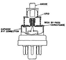
Fig. 16.28.—Lighthouse tube—cutaway view. Type 2C40.
