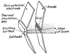
Fig. 15.24.—Pierce cathode structure for rectangular-beam parallel flow.
