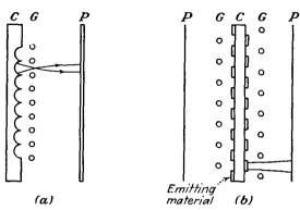
Fig. 20.26.—Electrode arrangements for reducing control-grid current.
