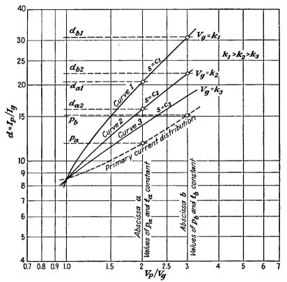
Fig. 9.24.—Effect of secondary emission on current division.
