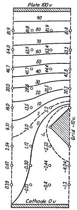
Fig. 5.11.—The potential field of a triode, calculated from the difference form of Laplace's equation, Eq. (5.44).
