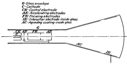
Fig. 15.12.—Structure of the postdeflection-acceleration tube.
