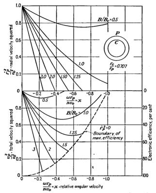
Fig. 18.22.—Total and radial electron velocity at the anode of a magnetron as a function of magnetic-flux density and angular velocity for a large ratio of cathode to plate radius.
