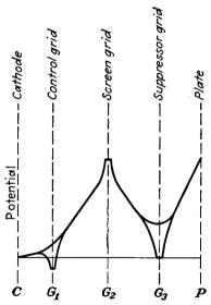
Fig. 11.1.—Potential profiles in a pentode.
