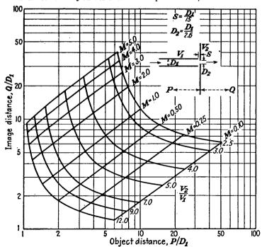
Fig. 13.45.—P-Q curves of a cylinder-aperture lens.
