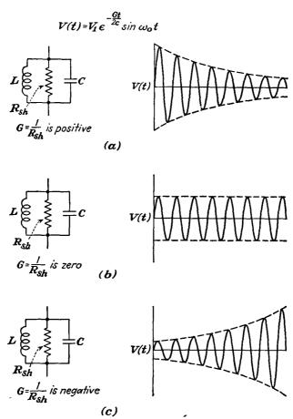
Fig. 17.32.—Transient response of an RLC circuit.
