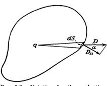
Fig. 5.3.—Notation for the evaluation of Gauss's law, Eq. (5.17).
