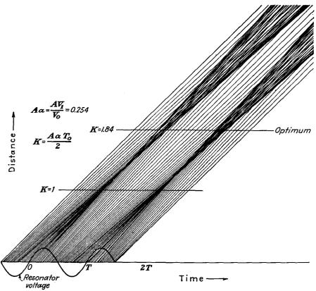
Fig. 17.6.—Distance-time diagram of a klystron amplifier.
