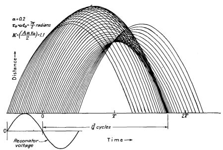
Fig. 17.30.—Distance-time diagram of a reflex-klystron oscillator.
