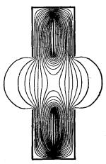
Fig. 13.16.—Potential field of an *Einzel* lens.
