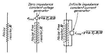
Fig. 12.2.—Equivalent circuits of a noisy resistor.
