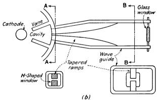
Fig. 18.2.—Output-coupling schemes for multicavity magnetrons.
