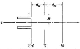
Fig. 15.4.—Idealized cathode-electrode configuration.
