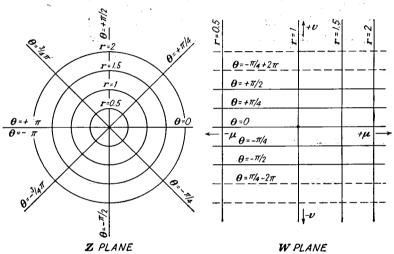
Fig. 5.17.—The logarithmic transformation,  $W = \ln_{\epsilon} Z$ .
