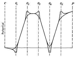
Fig. 20.15.—Potential profiles of a pentagrid converter.
