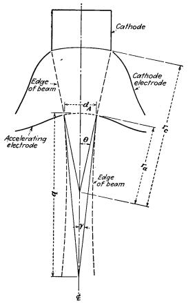
Fig. 15.34.—Diagram of a unipotential convergentbeam gun.
