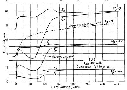
Fig. 10.2.—Plate-current-plate-voltage characteristics of a screen-grid tube.
