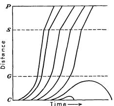
Fig. 16.26.—Distance-time behavior of electrons in a tetrode.
