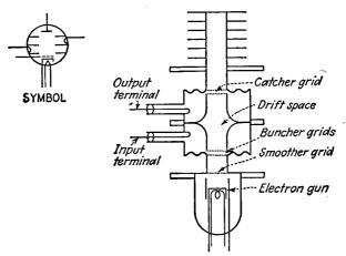
Fig. 17.16.—Structure of the two-resonator klystron amplifier.
