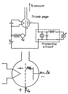
Fig. 21.19.—Basic circuit of the triode ionization gauge.
