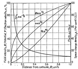
Fig. 8.3a.—Curves of potential, gradient, space-charge density, and velocity as a function of interelectrode distance in a space-charge-saturated plane diode, linear scales.
