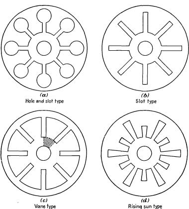
Fig. 18.1.—Various forms of multisegment anodes.
