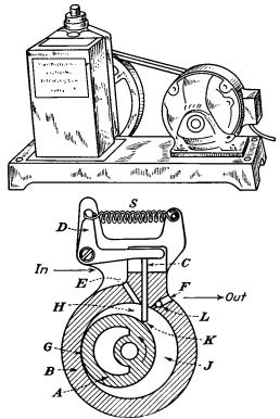
Pig. 21.26.—Diagram and picture of Cenco Hyvac pump.
