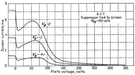
Fig. 10.4.—Screen-current-plate-voltage characteristics of a screen-grid tube.
