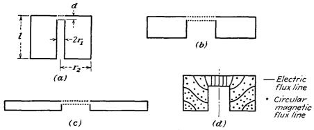
Fig. 17.2.—Reentrant cavity resonators.
