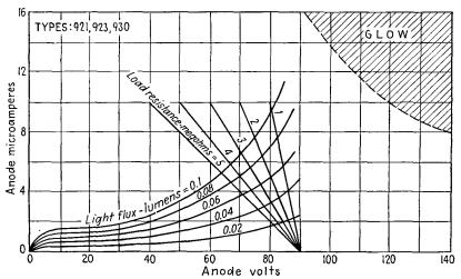
Fig. 19.10.—Current-voltage characteristics of a typical gas phototube.
