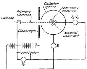
Fig. 4.14.—Apparatus for the measurement of secondaryemission characteristics.
