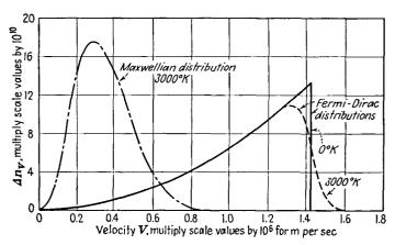
Fig. 4.1.—Maxwellian and Fermi-Dirac distribution of velocities in 1 cu mm of solid tungsten. The abscissa gives the relative number of electrons in a velocity increment of  $10^{-3}$  meters per sec in units of  $10^{10}$  electrons.
