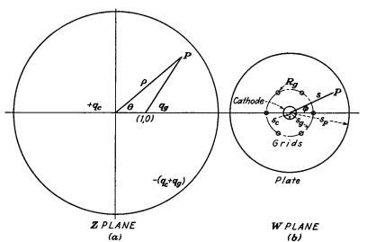
Fig. 7.5.—Elementary triode and equivalent cylindrical-electrode triode.
