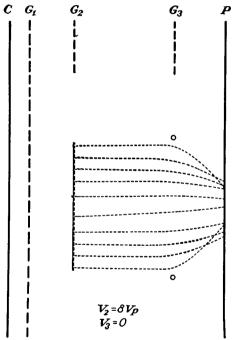
Fig. 11.15.—Focusing action of a large-pitch suppressor grid close to the plate of a pentode.
