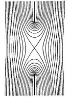
Fig. 13.14.—Aperture midway between plates at the same potential.
