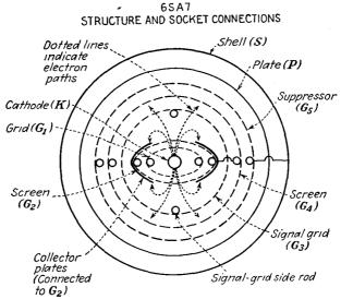
Fig. 20.16.—Structure of the 6SA7 special pentagrid converter.
