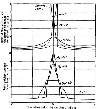
Fig. 17.9.—a (top) Current as a function of time along a bunched beam, for different degrees of bunching. b (bottom) Induced resonator current as a function of time for different intergrid transit angles. (After Black and Morton.)
