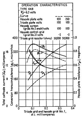
Fig. 20.5.—Conversion transconductance of a mixer tube.
