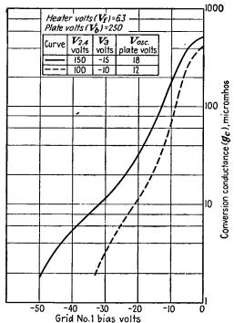
Fig. 20.14.— $g_c$ - $V_1$  characteristics of the heptode.
