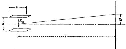
Fig. 6.2.—Electrostatic deflection of an electron beam. The electron enters the region of deflecting field at right angles to the field. The trajectory is parabolic between the plates.
