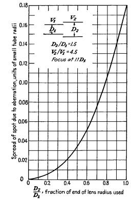
Fig. 13.57.—Minimum spot size as a function of aperture radius.
