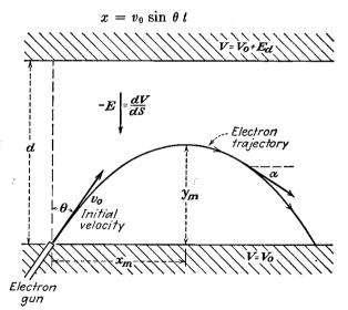
Fig. 6.1.—Parabolic electron trajectory in a uniform electric field. This case results from the injection of an electron with an initial velocity into a region where the electric field has a uniform retarding action.
